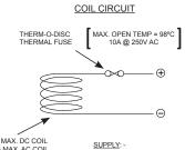
3W MAX. DC COIL 9VA MAX. AC COIL
