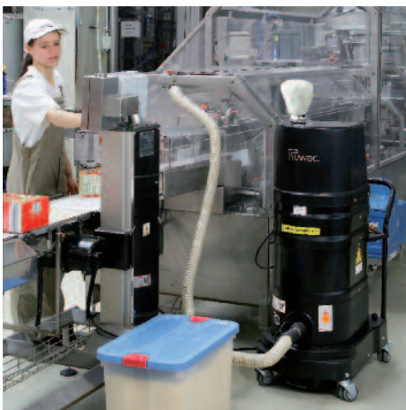
DS 1220 FS (fine dust) explosive dust in food production
