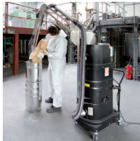
DS 1750 explosive dust, with extractor arm in the production of plastic
